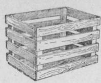
KNOCKED DOWN crates may be secured from the undersigned. These crates are made from good oak and chestnut lumber, the corner posts and sills being oak and slats chestnut, All material is sawed accurately, making construction easy, and general appearance of the crate neat,
