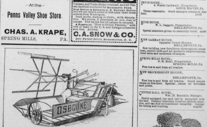
The Columbia Osborne Harvester and Binder is the acknowledged leader of harvesting machines. Two of its great features are the perfect swivel self-aligning boxes and the Osborne roller bearings. The Columbia is the only harvester and binder ever manufactured absolutely free of side draft and neck weight. The Columbia is an all steel binder.
