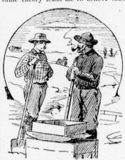
AT WORK AT CAPE NOME. (Separating Gold from Sand by Rockers and Cradles.)
