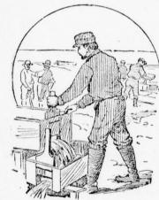
MINING AT CAPE NOME. (Washing Gold from Sand by Throwin Water Through Sluice Boxes.)
