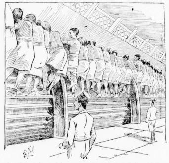
The whole machinery of the enormous prison at Rangoon, the largest in the east worked by human power generated by the treadmill seen in the picture, which accommodate 100 men at one time. The wrists of the prisoners are chained to a r, so that they cannot leave the mill until allowed to do so. If a convict is rectory, and will not tread, he simply falls down as far as his wrist irons will let him, while the ever-moving wheel barks his shins at each revolution.
