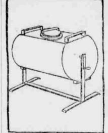
are placed in the receptacle, which is filled with water, the top screwed on and the cylinder revolved by means of a handle.
