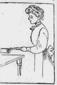
peal to all women who must work over the fire, being simple in construction and operation. Attached to the handie is a flat circular extension, which is slipped under the pan to be removed. Pivoted to handle is a lever, one end carrying a hook which drops over the edge of the pan. The other end rests against the handle. The lever prevents the pan from slipping. a small ring on the handle being slipped over the end, where it remains until the pan is safely removed and the lever disengaged.
