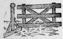
A Portable Fence. board will be needed in each panel. These panels may be 12 or 14 feet in length, well braced to keep the fence frin as to lengthwise motion. The cross-plete at the bottom of the upright should be long enough to keep the fence from the other mer. The construction is firm the other way. The construction is plainly shown in the illustration --American Agriculturist.
