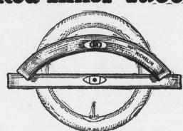
THIS picture illustrates an important difference in inner tubes. All tubes when inflated are ring-shaped like the tube in the background. But when deflated only the Michelin Tube remains curved. All others become perfectly straight.
