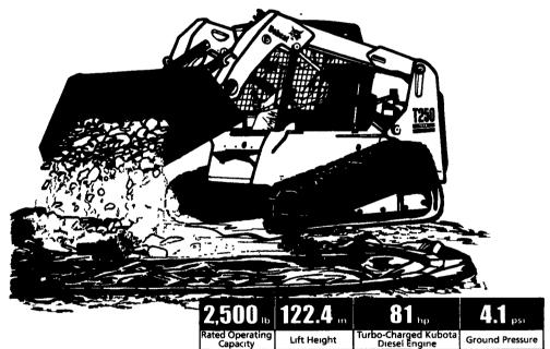
18-inch rubber tracks deliver extra traction, reduced ground pressure, low ground disturbance and excellent flotation. Extend your working season — get in earlier and finish faster, even on wet or muddy ground where other machines stop dead!
