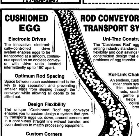
designed to fit 15° through 90° turns.
