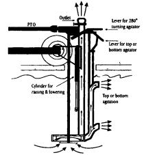
Available 6-8-10-12 ft. Dual agitation Hydraulic lift Simple controls
