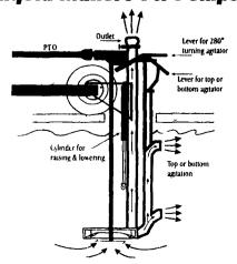
Trailer mounted mobility Dual agitation Hydraulic lift Simple controls
