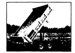
20" Sides 26" Front & Rear 3/16" Alum. Construction. 6 Ton Scissor Hoist, 10,000 # or 12,000 # GVW
