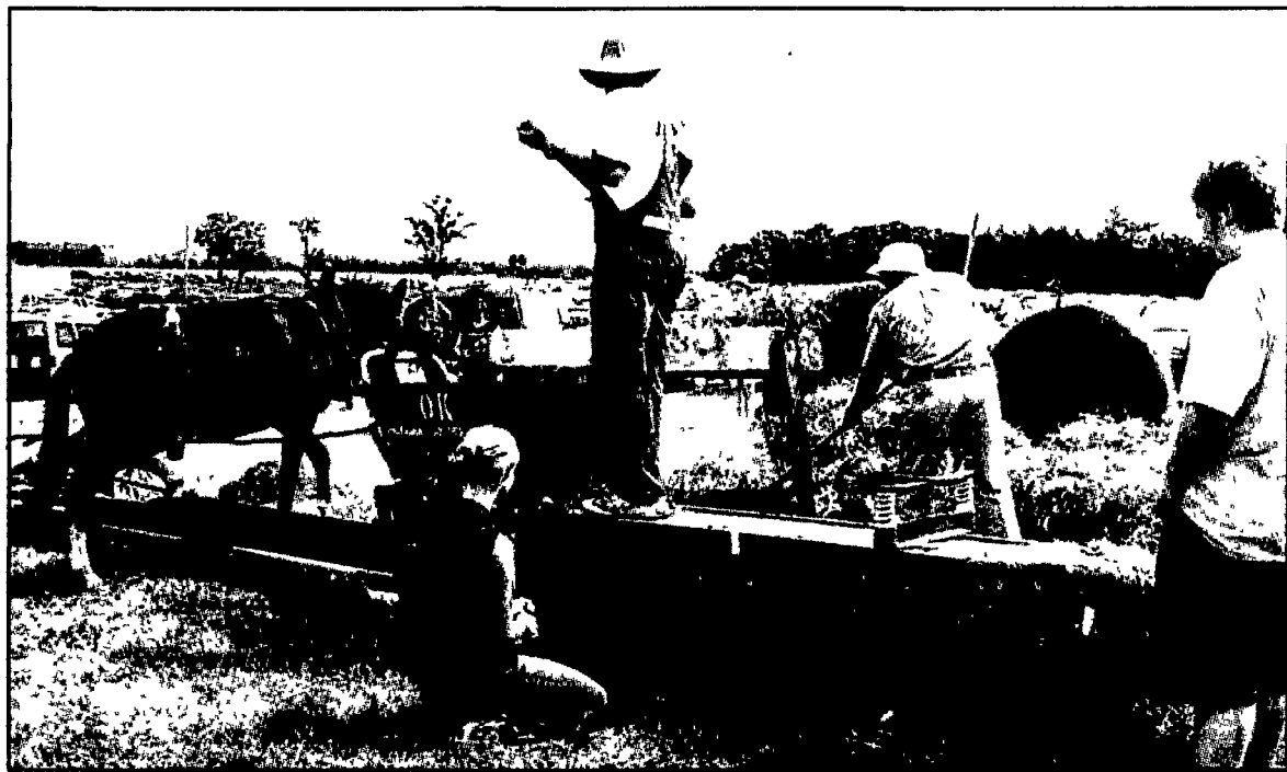
Three generations of the Robert Cowan family demonstrate a vintage horse-powered hay press. The 1905 stationary hay press shows how loose hay was pressed into rectangular bales weighing 100-120 pounds. A mule hitched to a 12-foot pipe sweep arm walks in a circle to drive a 16-foot-long plunger, which compresses the hay in a metal chamber. As the compressed hay emerges, long wires are placed around the bale by hand.
