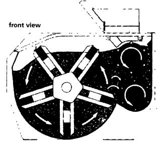
The large-diameter reel provides a gentle tumbling action and the two side augers produce an end-to-end blending action. This unique combination ensures faster mixing and unloading times, and a very thorough mix, even when mixing small batches.
