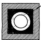
Chimtek Inner Liners are made of volcanic pumice and high-temperature refractory cements. Its round shape provides even temperature inside flue and contributes to efficient flow of smoke and flue gasses. The volcanic pumice in Chimtek liners adds considerable insulating value.
