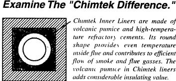
Chimtek Inner Liners are made of volcanic pumice and high-temperature refractory cements. Its round shape provides even temperature inside flue and contributes to efficient flow of smoke and flue gasses. The volcanic pumice in Chimtek liners adds considerable insulating value.
