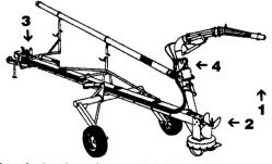
1-Highly articulated nozzle designed to slice and break the top crust from above the manure level as the propeller homogenises the liquid with the remaining floating chunks. 3-Hydraulic controls can be
