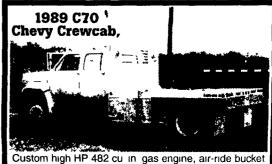
driver and passenger seat, pto & wetline, custom 9 ft aluminum stake body with swing-open end gates. trapdoor gooseneck hitch, chrome stacks Hydraulic brakes, 26,000 GVW Runs and looks great
