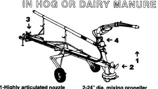
designed to slice and break the top crust from above the manure level as the propeller homogenises the liquid with the remaining oating chunks. 3-Hydraulic controls can be
