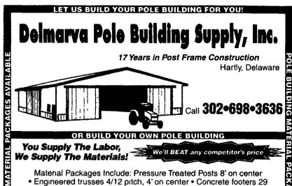
• Engineered trusses 4/12 pitch, 4' on center • Concrete footers 29 gauge painted steel siding and roof (25 yr. warranty, 19 colors to choose from) • 3'0" x 6'8" Steel service door with lockset 2"x4"'s every 2" on sides and roof • All trim and accessories included
