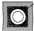
Chimtek Inner Liners are made of volcanic pumice and high-temperature refractory cements. Its round shape provides even temperature inside flue and contributes to efficient flow of smoke and flue gasses. The volcanic pumice in Chimtek liners adds considerable insulating value.
