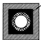
Chimtek Inner Liners are made of volcanic pumice and high-temperature refractory cements. Its round shape provides even temperature inside flue and contributes to efficient flow of smoke and flue gasses. The volcanic pumice in Chimtek liners adds considerable insulating value.
