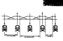
The pattern allows "back and forth" as well as "around and around" operation. The "truncated" pattern offsets inaccurate overlap problems, eliminating streaking.
