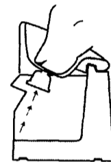
The JUG's Feed-Trap catches debris and keeps it out of the reservoir.
