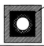
Chimtek Inner Liners are made of volcanic pumice and high-temperature refractory cements. Its round shape provides even temperature inside flue and contributes to efficient flow of smoke and flue gasses. The volcanic pumice in Chimtek liners adds considerable insulating value.
