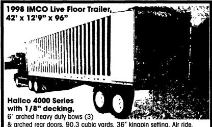
& arched rear doors, 90.3 cubic yards, 36" kingpin setting, Air ride, fixed tandem, Black tarp, cable style straps with ratchets, Black doors, plymetal split, double locks, 24.5 tires, Aluminum wheels (uni-mounts), Black aluminum side sheets, aluminum posts, aluminum top rail, aluminum floor crossmembers on 14.5" centers, Aluminum Bottom Rail, Actual scale weight ticket = 12,800 lbs.
