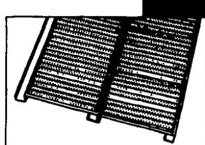
Brock's Perforated Plank Floors for aeration and drying
