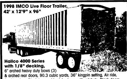
fixed tandem, Black tarp, cable style straps with ratchets, Black doors, plymetal split, double locks, 24.5 tires, Aluminum wheels (uni-mounts), Black aluminum side sheets, aluminum posts, aluminum top rail, aluminum floor crossmembers on 14.5" centers, Aluminum Bottom Rail, Actual scale weight ticket = 12,800 lbs.
