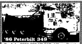
Tri-Axle, 3306-300 HP CAT, 18k on Front, 46k Rears, 8LL Trans, PS, AC, Auto Tarp, New Drum & Brakes, Good Tires, Setup For Trailer With Air Brakes, Great Shape,
