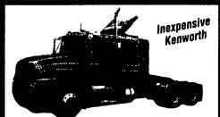
1988 Kenworth T600, 63" Flat Sleeper Cat 3406B 425 HP w/Jake Brake, Kenworth 8 Bag Air Susps., Eaton 12# Front & 38# Tandem Axle, Fuller 13 Speed w/OD Trans, Alum. Wheels Stock #508617 As Is \$10,500
