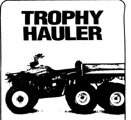
New! SPORTSMAN 6X6 • Powerful Polaris 500, 4-valve 4-stroke, liquid-cooled engine • Automatic transmission (PVT) • Thumb-switch engage, true 6-wheel drive • MacPherson strut long-travel (6.7") front suspension • Rear suspension. progressive rate center swing arm, 6 5" of travel; rear swing arm with scissor stabilizer, 7.5" of travel • All-wheel hydraulic disc brakes • Composite rear dump box, hinged for easy unloading (800 lb capacity)
