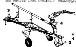
designed to slice and break the top crust from above the manure level as the propeller homogenises the liquid with the remaining floating chunks. 3-Hydraulic controls can be
