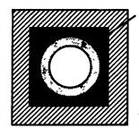
Chimtek Inner Liners are made of volcanic pumice and hightempertature refractory cements, Its round shape provides even temperature inside flue and contributes to efficient flow of smoke and flue gasses. The volcanic pumice in Chimteck liners adds considerable insulating value.
