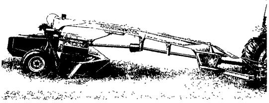
For greater maneuverability and higher efficiency, nothing beats the Model 1431 Discbine® disc mower-conditioner from New Holland. If features a 13' cutting width, and operates at high ground speeds in wet, heavy grass without plugging. Fire anthills and gopher mounds won't stop the new Model 1431 either. Outstanding features include:
