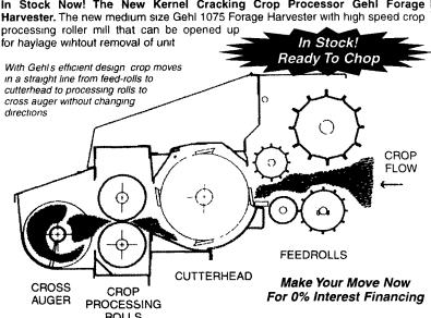
Located directly behind the cutterhead cylinder, the Crop Processor features a pair of high-speed grooved rolls that crack kernels, break up the cob and shred the stalk material
