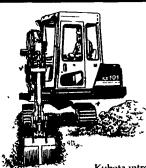
Kubota introduces the KX-Series mini-compact excavators from 22 2 HP to 42 7 HP, featuring Kubota's "Power Up" hydraulic system
