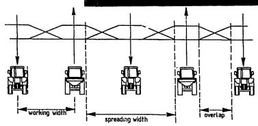
The pattern allows "back and forth" as well as "around and around" operation. The "truncated" pattern offsets inaccurate overlap problems, eliminating streaking.
