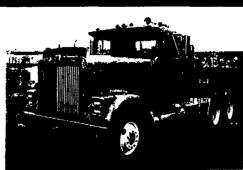
87 International, 4700, Cummins L10 300 HP, 9 Speed, 190 W.B. 12/40 Axles, Air Ride Susps.
