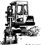
Kubota introduces the KX-Series mini-compact excavators from 22 2 HP to 42 7 HP, featuring Kubota's "Power Up" hydraulic system that increases digging performance and traveling speed
