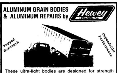
through engineering, not strength with bulk. For example, a 16' grain body with tailgate and 48" sides weighs only 1490 lbs. complete. We'll build you any length or any side height up to 60".
