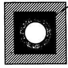
Chimtek Inner Liñers are madeof volcanic pumice and hightempertature refractory cements, Its round shape provides even temperature inside flue and contributes to efficient flow of smoke and flue gasses. The volcanic pumice in Chimteck liners adds considerable insulating value.
