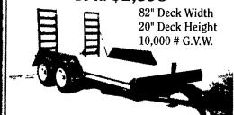
6" Channel Tongue and Main Frame Choice of 2 5/16" Coupler or Pintle Ring 7000# Drop Leg Jack Treated Yellow Pine Floor Stake Pockets fits standard 2x4's heavy Tie Rail with Reflective Tape
