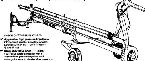
Hydraulic Controls — trailer, horizontal and vertical movement and agitate/fill valve are easily operated from the tractor
