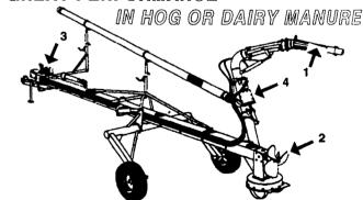
1-Highly articulated nozzle designed 2-24" dia. mixing propeller providing to slice and break the top crust from above the manure level as the propeller homogenises the liquid with the remaining floating chunks.
