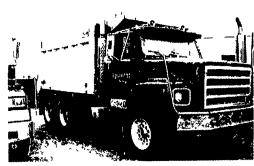
1979 IH S2600 15' Dump Body, NTC-400 Eng, Jake Brake, 13 Speed Trans, 4 44 Rear Ratio
