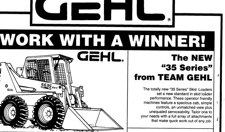
5635 • 60 h.p. oil-cooled diesel engine • 80 h.p. turbocharged oil-cooled diesel (opt.) • 1800 lb. SAE lift capacity • 42" wheelbase
