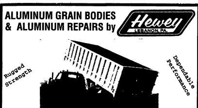
These ultra-light bodies are designed for strength through engineering, not strength with bulk. For example, a 16' grain body with tailgate and 48" sides weighs only 1490 lbs. complete. We'll build you any length or any side height up to 60".
