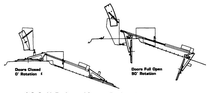
A.O. Smith Engineered Storage Products has developed a way to avoid the strenuous and unpopular job of climbing to open and close the doors on your Harvestore structure: *The Push Button Fill Doors™ system!*
