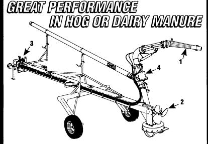
to slice and break the top crust from above the manure level as the propeller homogenises the liquid with the remaining floating chunks.
